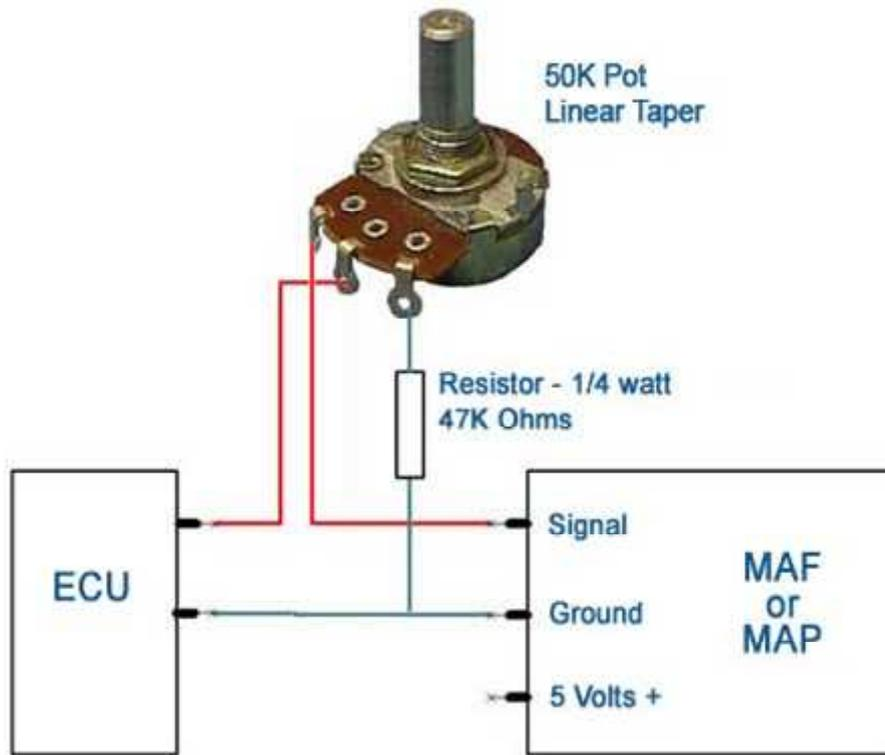
**Note:** The MAF is often combined with an Intake Air Temperature sensor so may have more wires than shown here. The 5 Volt wire is not shown in the diagram because we don't do anything with it. But it is left in place. Do not cut it. Find the signal wire by revving the engine and finding the terminal that changes voltage.
